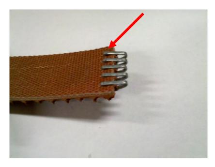
Now flip the tread back over so the tread is exposed, and finish tapping the Alligator Clip tight.
