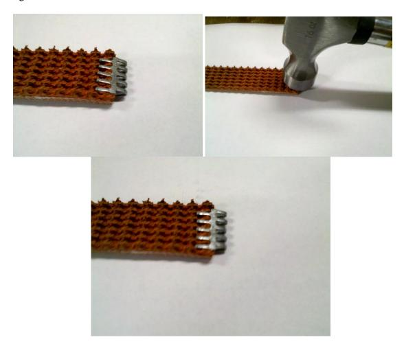
Do the same thing to the other end of the tread, wrap it around your wheel, and slide the pin between the clips. (If you are doing this on a placation wheel, you will need to loosen the wheel to get the tread to fit, after you do this step be sure to tighten the wheel halves together)
