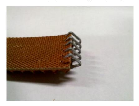
Use a hammer to tap down the longer points into the tread, use a motion more inline with the points.
